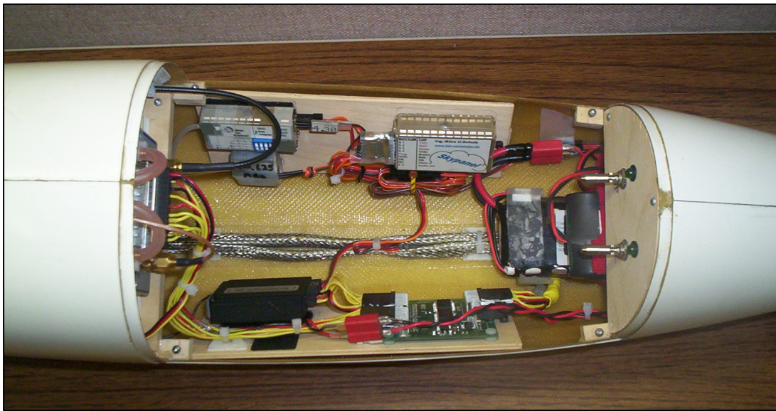
Figure 6: System Setup. Boxes CW from bottom right are: RxMux, RC Receiver, Piccolo autopilot, Skymelody system, and batteries.
